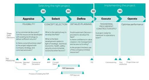
Figure 1.4 The stage-gate process and the FDP
